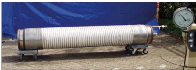
Ambient burst test on prototype Multi-LNG White 16"
