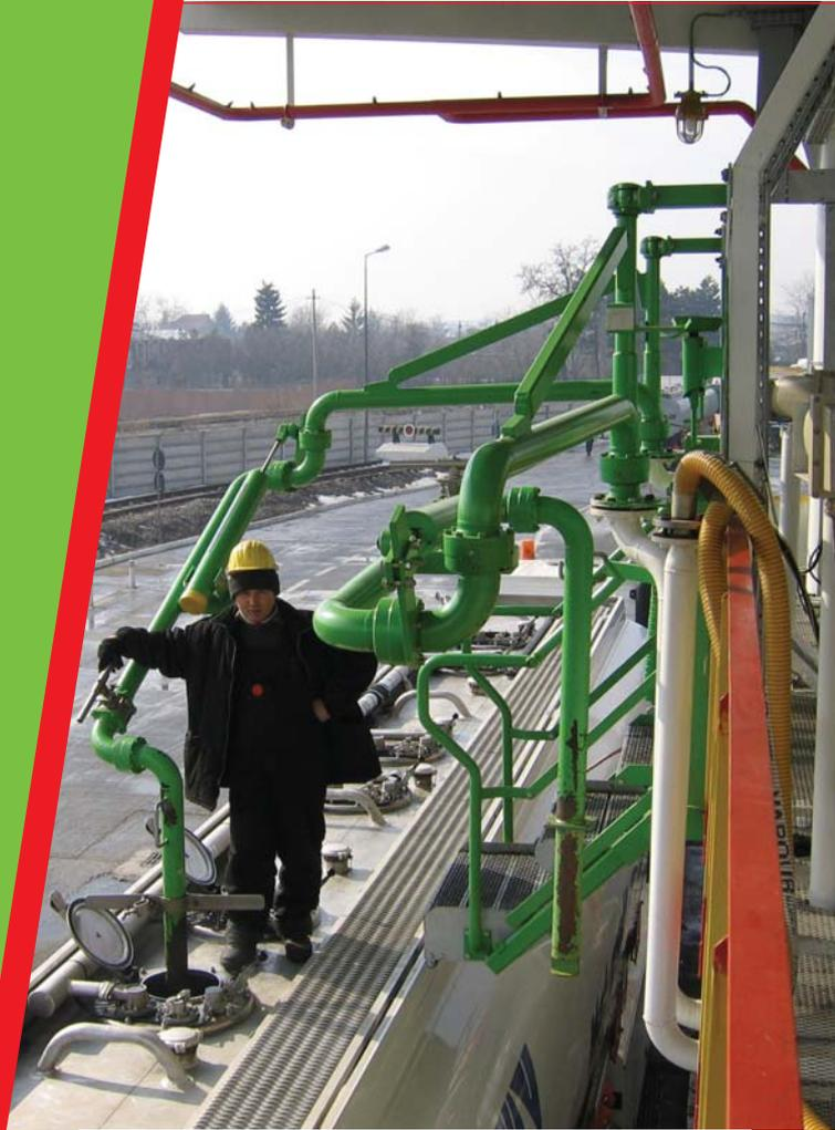
KANON top loading arms are specially designed to suit both open filling of a wide range of products across all industry sectors or closed filling of the type of highly aggressive liquids associated with the chemical and petrochemical industries.
