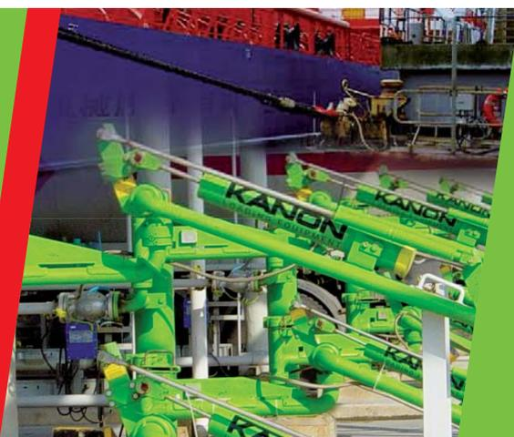
Loading equipment for marine, road, and rail tankers
