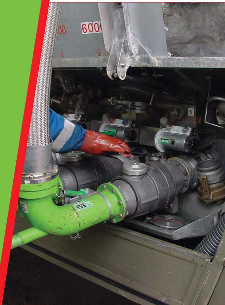
KANON cross-over bottom loading arms allow simultaneous connecting and filling of up to seven product lines with vapour return.
