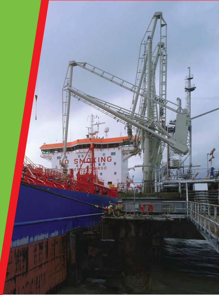
The transfer of all fluids and liquefied gases, into the smallest barge or the largest crude carrier may be safely and dependably accomplished using a KANON Marine Loading Arm system.
