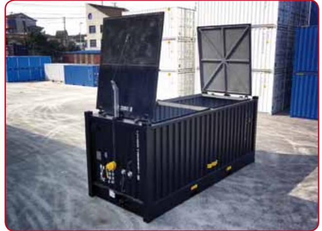
The melter is insulated with latest Nano Technology and comes with temperature control. Optional is a Thermostat that will have further energy savings.
