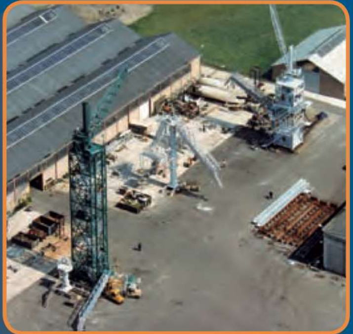
All Verhoef Access Systems are shop-erected and fully tested before delivery, through which a quick commissioning of the equipment at site is guaranteed.
