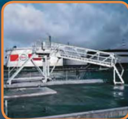
Riding ladder, hydraulically operated. Antwerp - Belgium
