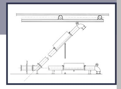
swing joint design. This design eliminates the unbalanced lading of a conventional swing joint. CTS is more than willing to design a floating suction line or a skimmer unit on the basis of using your preferred supplier for the important swing joints required as part of the assembly.
